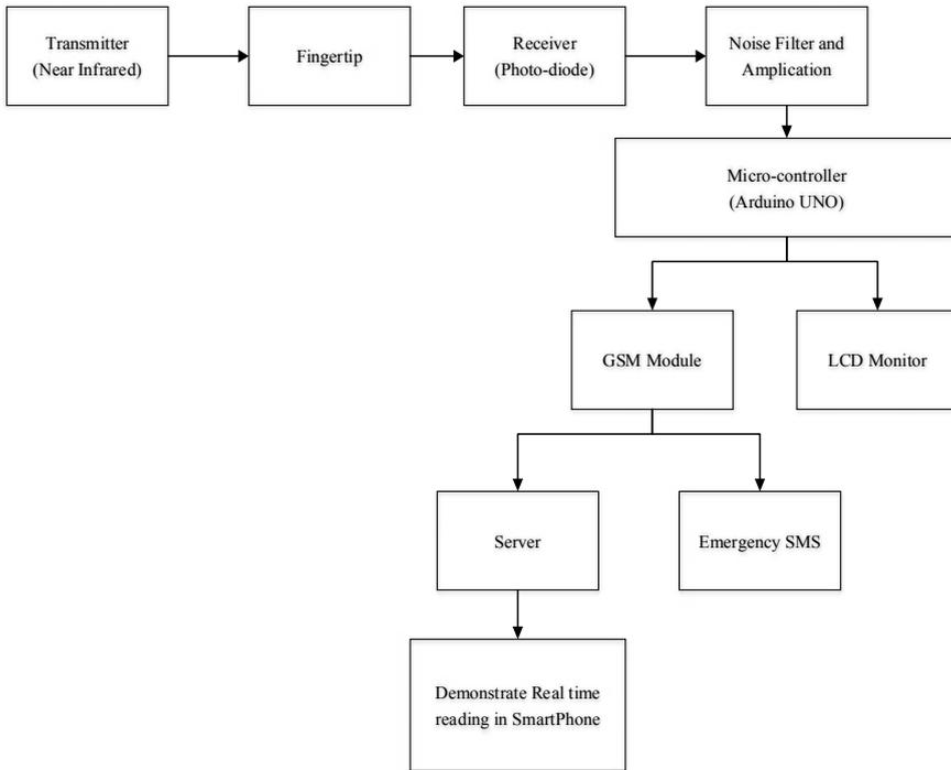
**Fig. 1** Proposed block diagram of non-invasive blood glucose monitoring system
