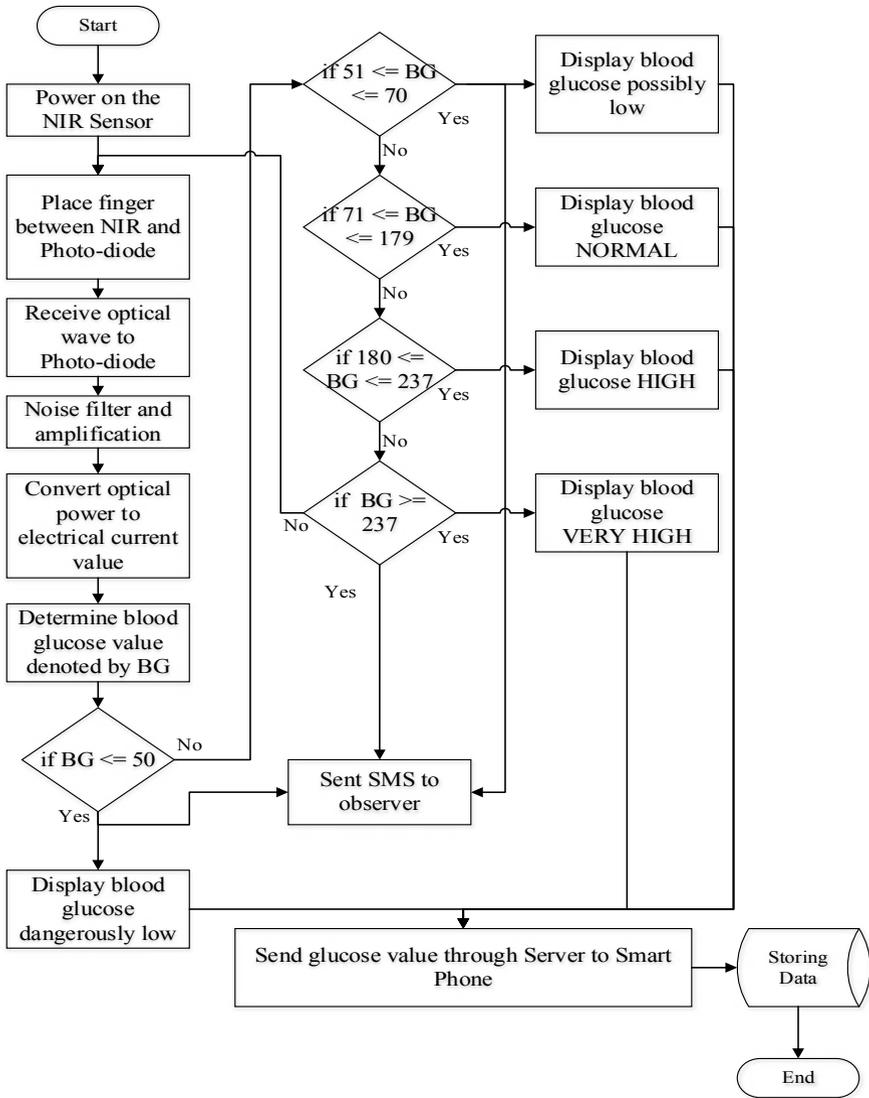
Fig. 3 Flowchart of working procedure of the proposed system
