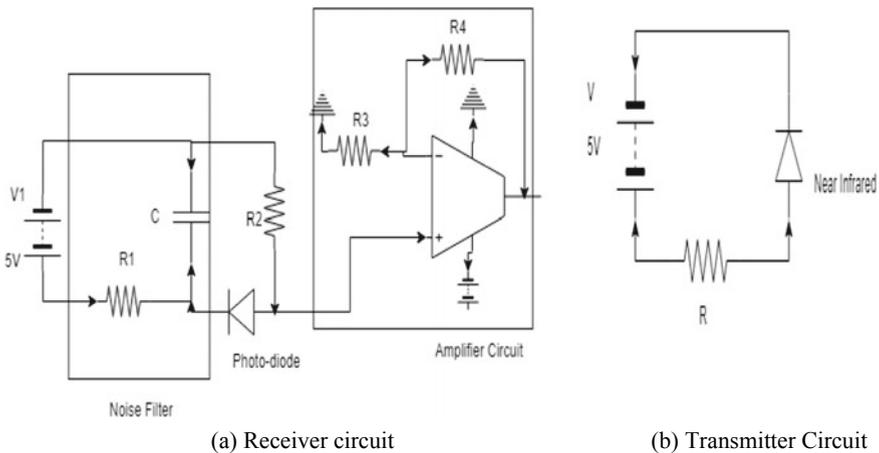
Fig. 4 Schematic diagram for measuring blood glucose
