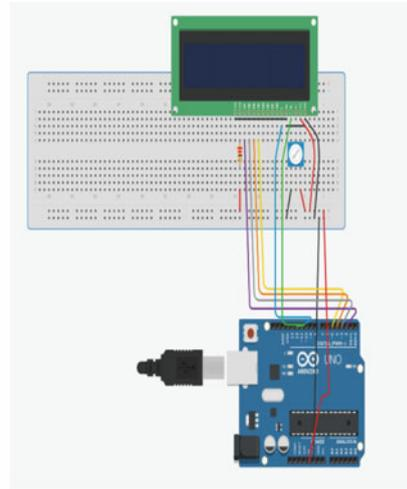
(b) LCD display circuit
