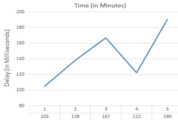
**Fig. 4.** Effective Latency in Normal Jitter Buffer.
