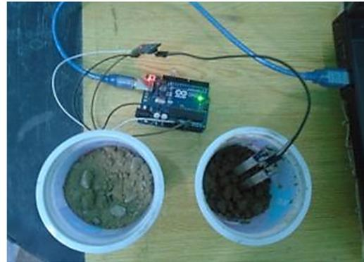
Fig. 7. Test setup for soil moisture level
