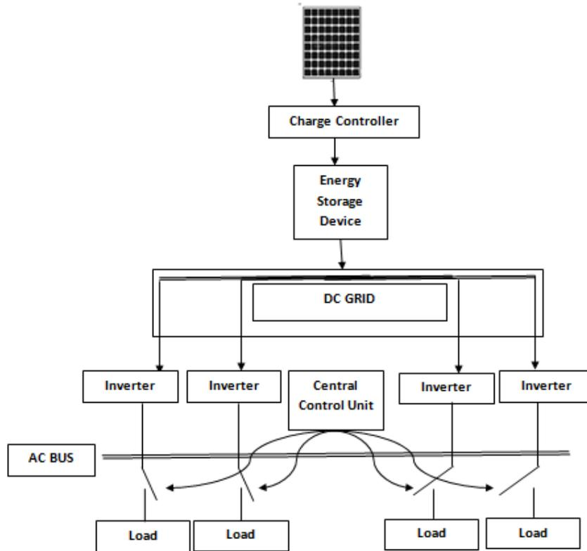
Fig. 4. Prototype of DC grid.
