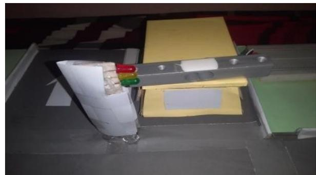
Fig. 5. Collision Detection using Load Cell.
